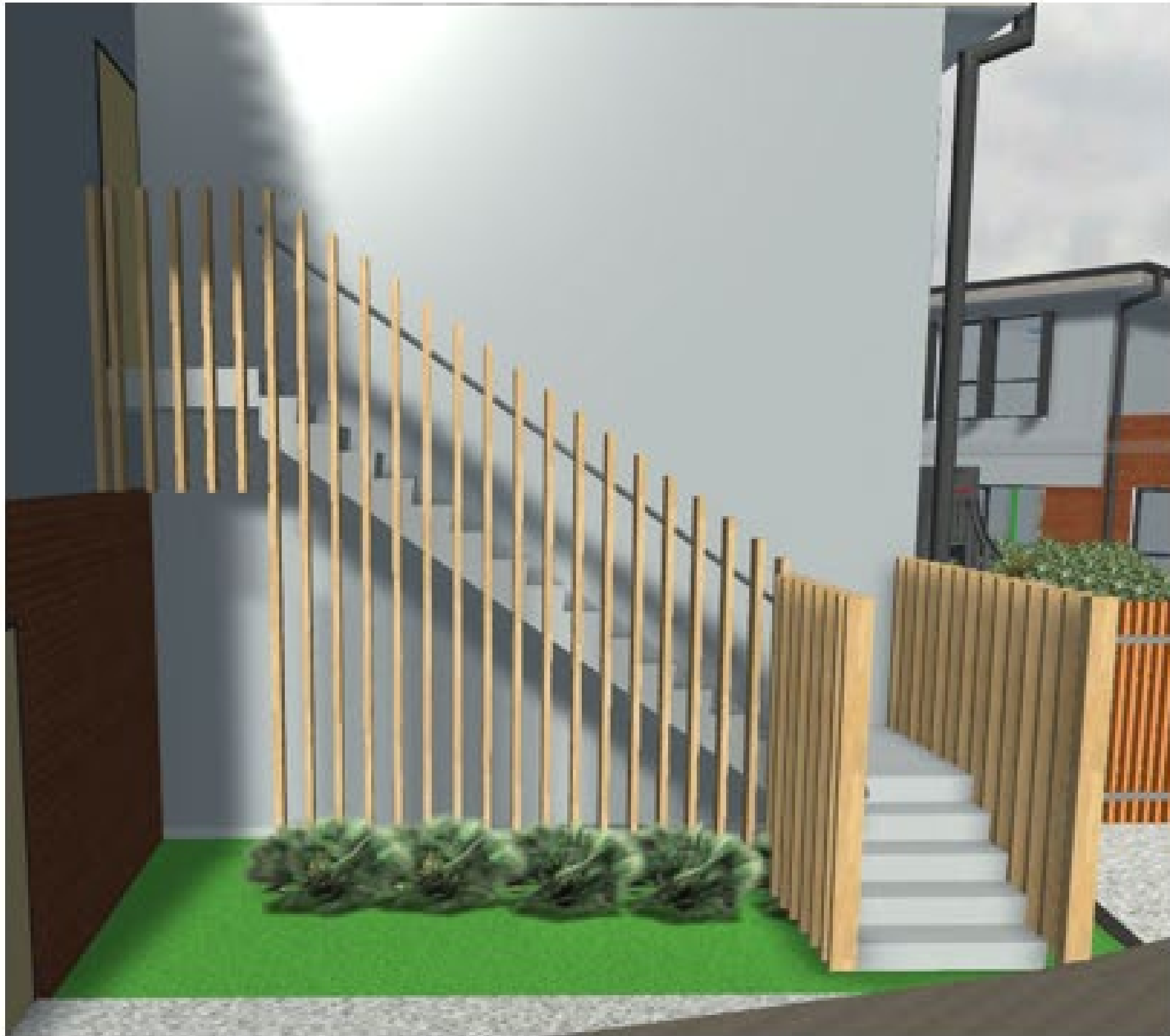
ALUMINIUM (TIMBER LOOK) BLADES – TYPICAL FOR EXTERNAL STAIRS
