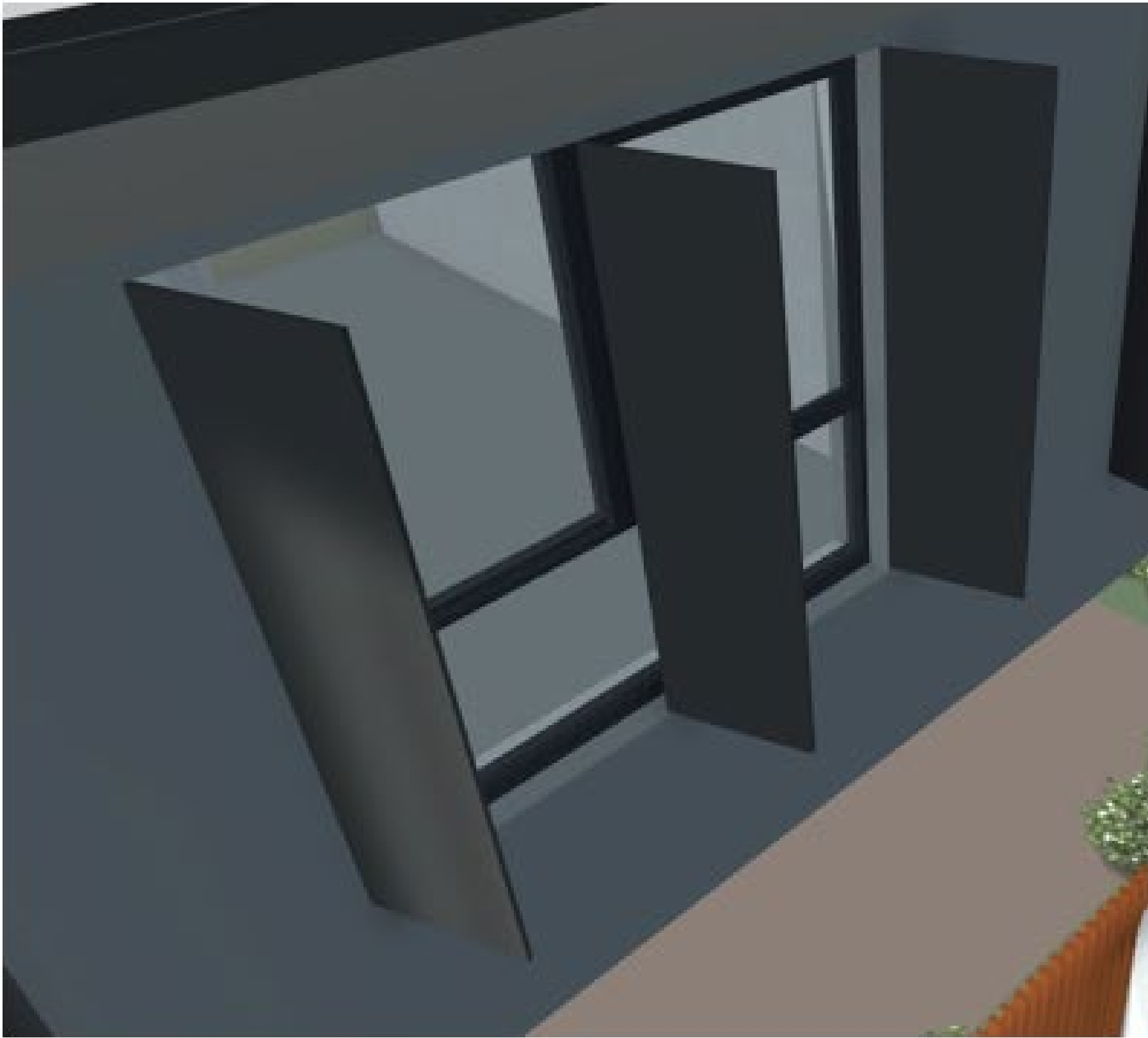
600-700MM PERFORATED ALUMINIUM BLADES TO MATCH WINDOW HEIGHTS
